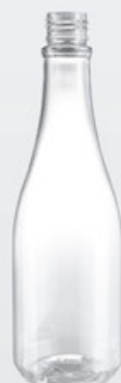
BT24-G360 容量Capacity: 360ml 口径Neck: 28/410 克重Weight: 36g 尺寸Size: Ø63.5*H205.8mm
